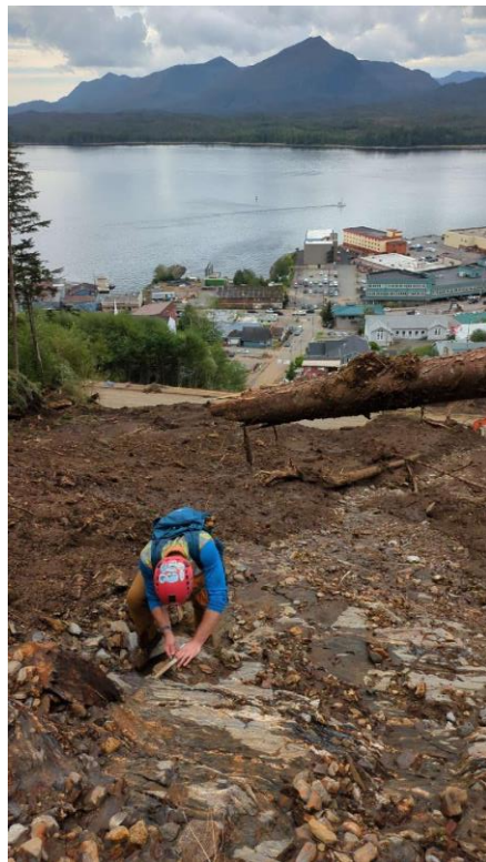
B: 3rd Avenue Landslide, Point 5, phyllite exposure in recently developed drainage channel.
