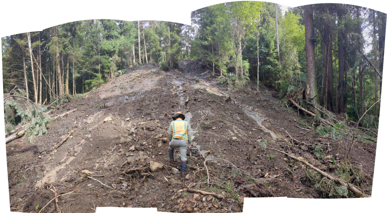
A: 3rd Avenue Landslide, Point 35, glacial till exposure in recently developed drainage channel.
