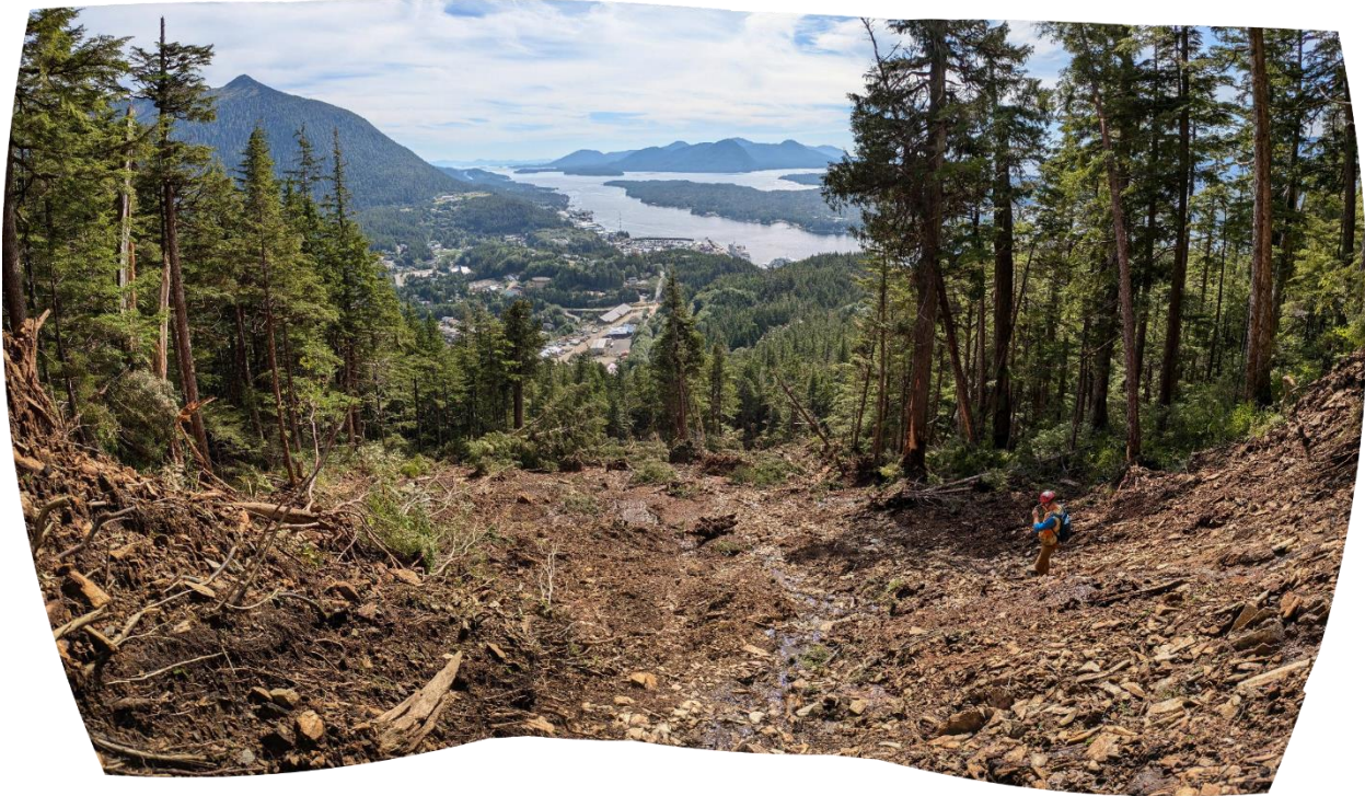
A: Copper Ridge Landslide, Point 1068, Upper Zone, thin colluvial deposits, looking southeast.
