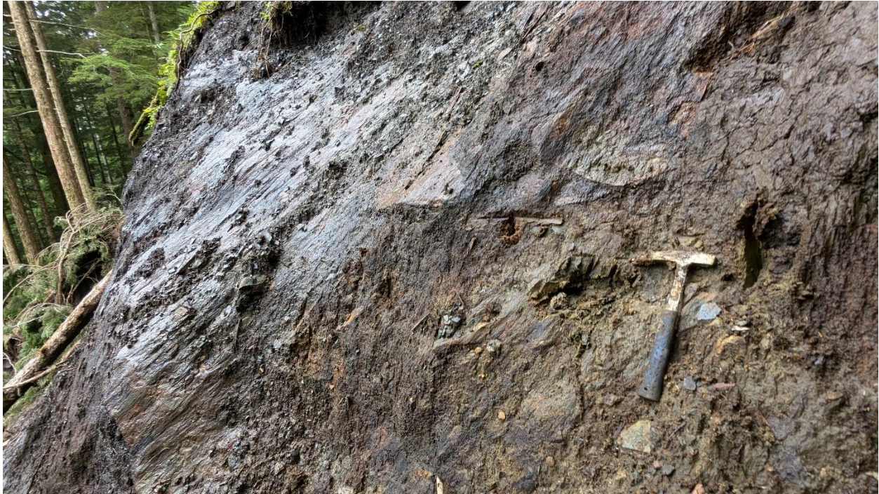
A: 3rd Avenue Landslide, Point 46, exposure of decomposed phyllite with slickensides.
