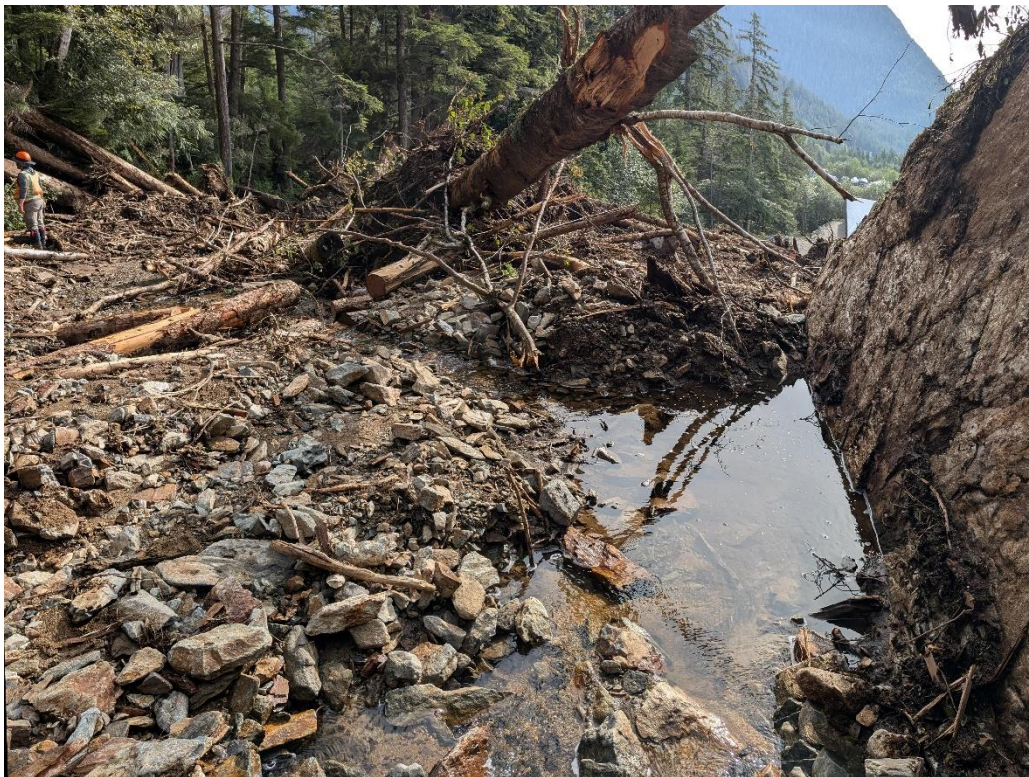
B: Copper Ridge Landslide, Point 1018, Lower Zone, drainage channel diversion at base of steep slope near landslide toe.
